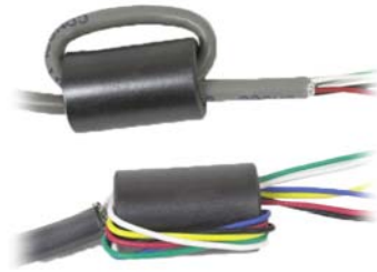
Figure 2-12: Installing the Ferrite Cores
