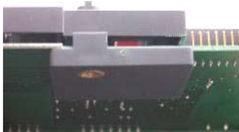
Figure 2-60: Attaching the Plastic Bottom Sealing Plate
