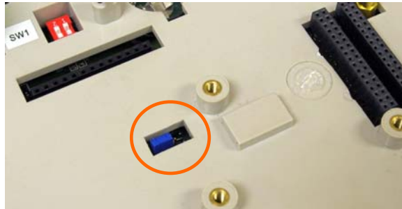
Figure 2-52: W1 Millivolt Jumper Location, Main PCB Cover Installed
