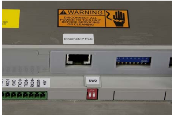
Figure 2-47: EtherNet/IP Label Placement on Panel Mount Terminal
