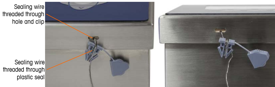
Figure 2-59: Harsh Enclosure Seal Threaded and Ready to be Closed – Standard Orientation (left) and with Panel Reversed (right)
