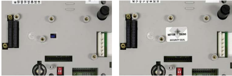
Figure 2-63: W1 Millivolt Jumper – Unsealed (left) and Sealed (right)
