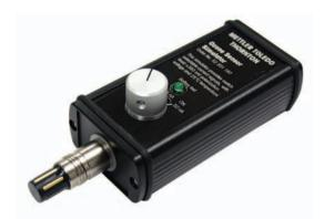
Startup of Mettler-Toledo Thornton ozone instrumentation can be expedited using the Ozone Sensor Simulator. The Simulator takes the place of the sensor and provides ozone and temperature signals without the need for ozonation and sensor polarization. The Simulator allows measurement verification (except for the sensor) ahead of treatment system startup.
