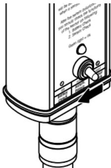
By pushing the switch **to the left** to the position "**1 – Battery check**", the O<sub>2</sub> Sensor-Master will control the polarization voltage. If the green LED lights up than the battery is still ok and delivers the correct polarisation voltage. If not, the battery must be changed (see section 2.3). If after a battery change, the LED does not light up you will have to return it to your METTLER TOLEDO dealer.
