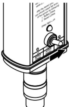
Expose the sensor (connected to O<sub>2</sub> Sensor-Master) to the air. By pushing the switch **to the right** to the position "**2 – Sensor check**", the O<sub>2</sub> Sensor-Master checks whether the electrode current for air measurement delivered by the sensor is within the admissible range (40 to 100 nA for an InPro 6800; 250 to 500 nA for an InPro 6900; 2500 to 6000 nA for an InPro6950).
