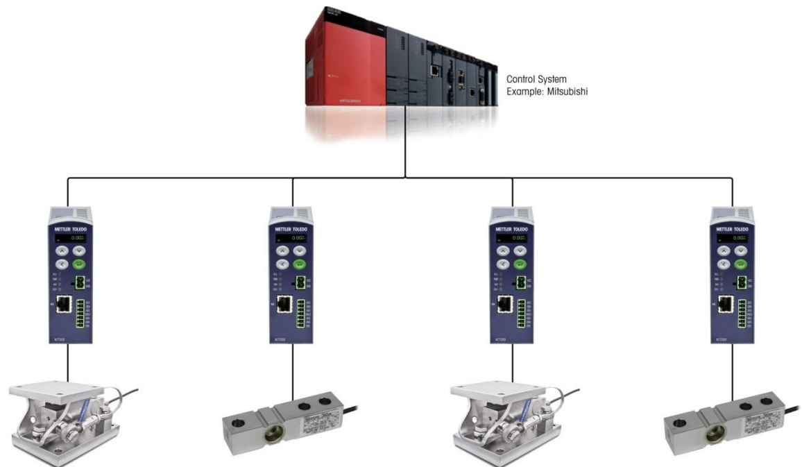
Figure A-1: Overview of a Control System
