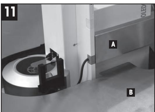
**CAUTION:** When adjusting the height of the tables, the cover [A] and the metal sheet [B] must not touch, otherwise the balance might get damaged.
