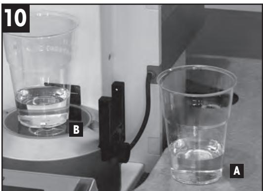
Check installation with two cups of water: Slightly shake the working table [A]: The water surface on the balance table [B] should remain still.
