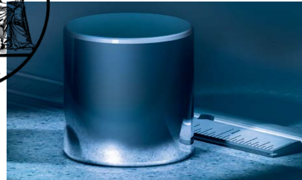
International Prototype Kilogram (IPK) at BIPM, a cylinder made of 90% platinum and 10% iridium.
