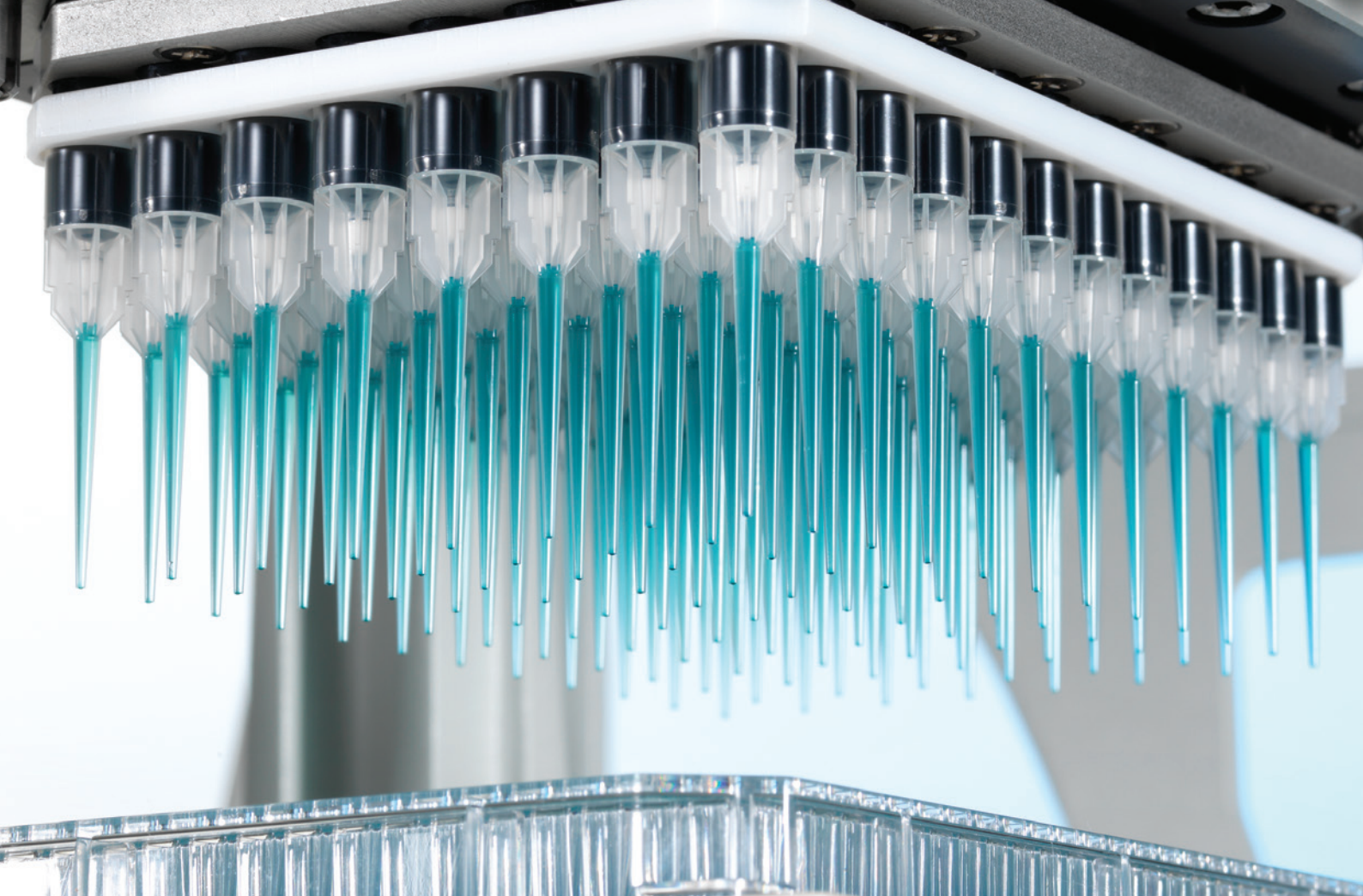
20 \mu L Liquidator 96 is accurate to 0.5 \mu L
