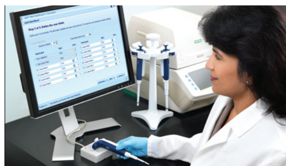
Optional RFID Reader works with all Rainin RFID-enabled pipettes, and interfaces with METTLER TOLEDO's LabX™ Direct Pipette-Scan™ calibration check.
