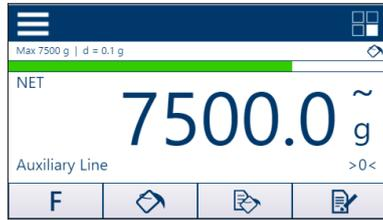
1. Press **F** in the main screen to enter into the Application screen, then press Factor Value Setting **F** Factor Value Setting.
