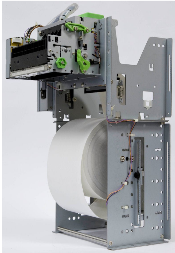
Figure 2-17: Properly Loaded Paper Roll
