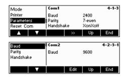
The current Baud Rate, Parity and Handshake settings are displayed on the screen. Press « >>> » and ...
