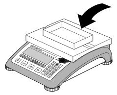
Place the **empty** weighing container or packaging on the scale and then press the  $\leftarrow$ T $\leftarrow$ » key briefly, or press the  $\leftarrow$ PT» softkey if a **known tare** weight has already been established.
