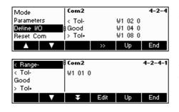
Go to "Vision Setup  $\rightarrow$  COMMUNICATION  $\rightarrow$  COM X  $\rightarrow$  Define I/O and then press «  $\Longrightarrow$  » to change settings for the I/O relay box.
