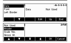
Choose "Date" to define the desired information for the line that was chosen. A detailed list of all functions can be found on the menu diagram (see Chapter 5.3.4 "COMMUNICATION  $\rightarrow$  Def. Heading Line  $\rightarrow$  Template 1-5  $\rightarrow$  Edit  $\rightarrow$  Line 1-23  $\rightarrow$  Data").
