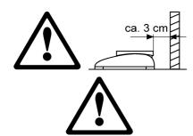
If the **power cord** is damaged, the scale must no longer be operated. Therefore check the cable regularly and ensure that a free space of about 3 cm is left at the rear of the scale, so that the cable is not kinked too severely.
