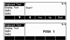
In order to check if all the keys are functioning properly, press  ${\tt «Yes»}$  to start the keyboard test.
