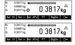
Wait until the stability detector (a small ring at the left edge of the display) disappears, then...
