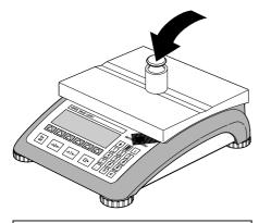
After choosing the calibration weight, place the weight on the weighing pan and then press the  ${}^{\diamond}$ **OK** ${}^{\diamond}$  softkey.
