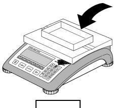
Place the **empty** weighing container or packaging on the scale.
