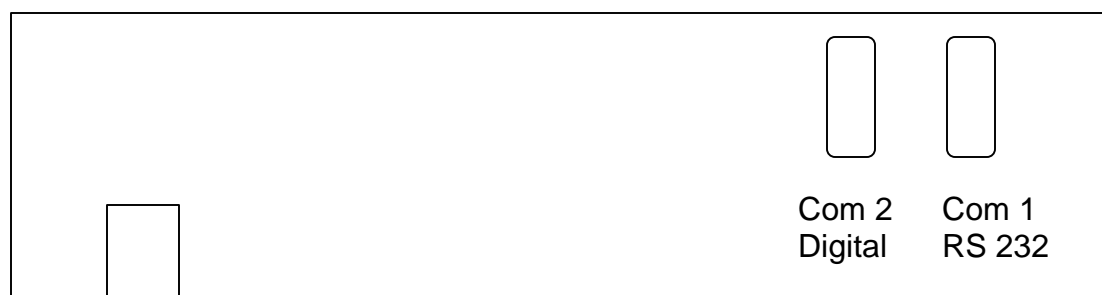
Connector plate on rear of scale / terminal.
