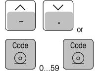
Selection of the desired storage position of a new program (Display: -n- for empty positions, otherwise program name). The positions are shown by the DeltaTrac.
