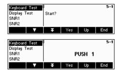
In order to check if all the keys are functioning properly, press  ${\it \bf «Yes.}{\it \bf »}$  to start the keyboard test.
