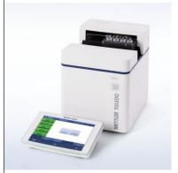
Sample loading is easily automated with the FillPalMini, which pumps the sample safely into the flow cell. It can also be used for sample recovery and cuvette cleaning. Multiple samples are efficiently analyzed using the Plug & Play CuvetteChanger, including the measurement of sample series on the UV5Bio.
