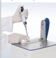
The UV5Nano is two instruments in one for micro-volume and cuvette based measurements. Once the arm is at 90 degrees position the measurement surface can be easily accessed with a pipette from either the left or the right side. The curved lid on top of the instrument allows convenient positioning of the operator's hand to securely guide the pipette tip.
