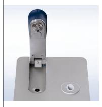
Micro-volume UV/VIS measurement is the method of choice if small sample amounts or if high absorption samples need to be measured. Only 1  $\mu$ L of sample is required for reliable measurements. The pure sample is pipetted on the measurement surface and the arm is automatically locked to a precisely defined pathlength. Measurement errors are avoided as the sample does not need to be diluted.
