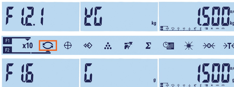
Figure 1-7: Unit Switching: Kilograms to Grams
