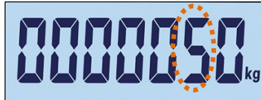
Figure 2-4: Changing Numerical Values, Digit in Focus Blinking
