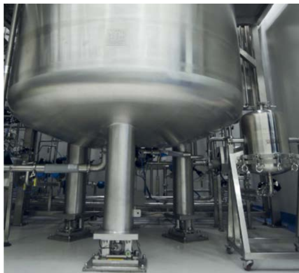
Lower section of the reactor mounted on flexible compression weigh modules
