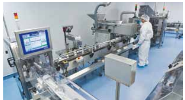
In-process control systems help record and analyze process data to ensure consistent quality
