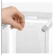
Quick to dismantle Remove, clean and put back all of the QuickLock draft shield glass panels in just a few simple steps, without tools and without moving the balance.
