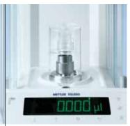
PipetteCheck Balance and stand-alone pipette check-station combined, for checking pipette accuracy.
