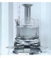
Density Kit Density determination becomes easy with METTLER TOLEDO's density kit for analytical and precision balances.
