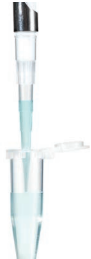
Dispensing onto liquid surface
