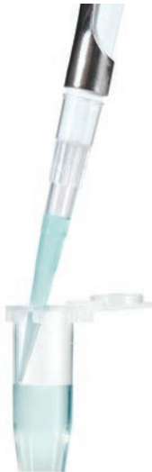
Dispensing against vessel wall
