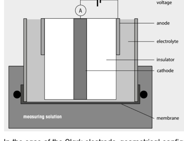
In the case of the Clark electrode, geometrical configuration is very important. In particular, the thickness of the electrolyte film between the cathode and the membrane must be within narrow tolerances so as to ensure good linearity and a low zero current (current in a nitrogen atmosphere). The figure above exemplifies the principle of the design of a Clark-type oxygen electrode.
