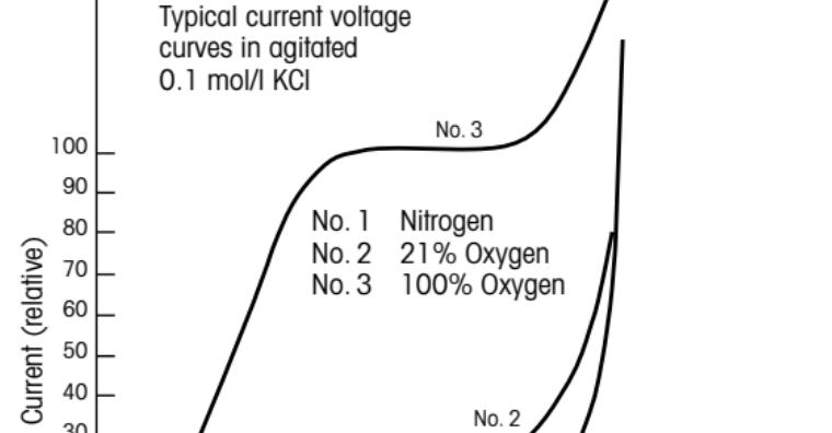
The polarization voltage should remain as constant as possible. Besides a constant source of voltage the following prerequisites must be met:
