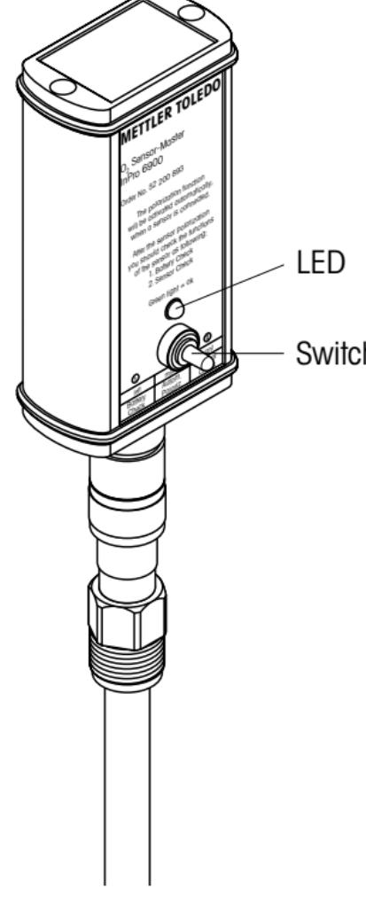
As soon as the sensor is connected to the O<sub>2</sub> sensor master, the polarization function is automatically activated. Please note: if the sensor was disconnected from the transmitter for longer than 5 minutes, the sensor must be polarized first (polarizing time see "Section 5.1") to get representative test results.
