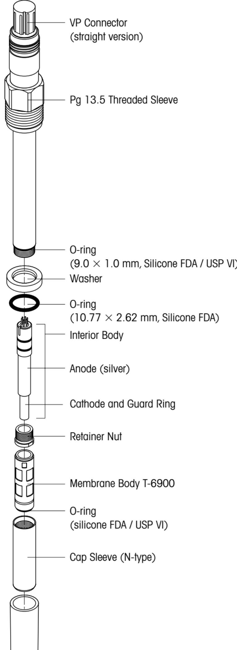
METTLER TOLEDO DO sensors are supplied with fitted membrane body filled with electrolyte and covered with the watering cap and have been checked for proper function.
