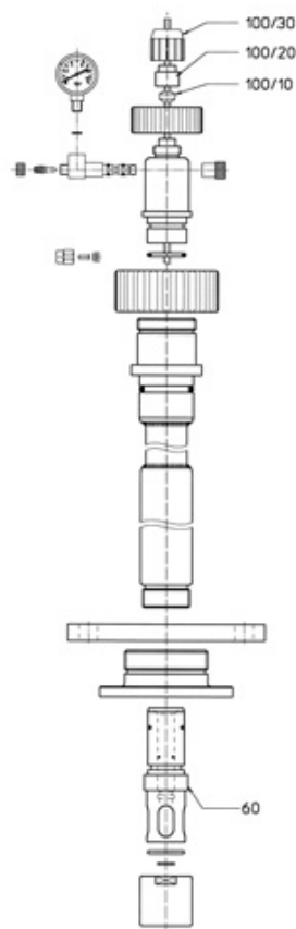
Removal of electrode from InFit 763e housing (PVDF plastic version).
