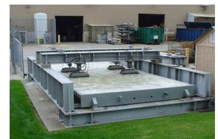
100% of the CLC is applied to the module up to 2 million times . Any design flaws that occur will be adjusted and the new design will go back through the full testing process
