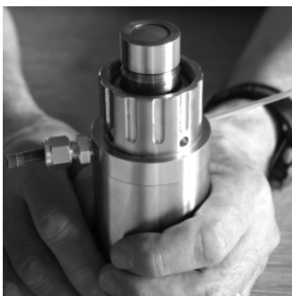
Fig. 1: Hold sensor in upside down position during maintenance e.g. MembraCap change
