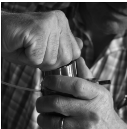
Fig. 6: Screwing on the new MembraCap
