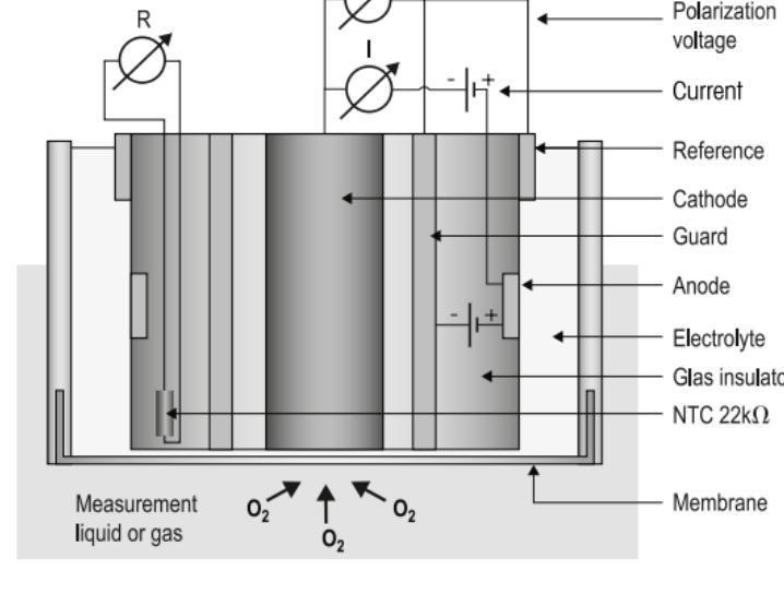
As a consequence of the reaction at the cathode and the anode, a current flows between cathode and anode (4 electrons per oxygen molecule), which is proportional to the oxygen partial pressure at the cathode.
