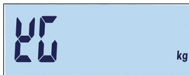
Figure 3-28: Primary Units Setting Screen
