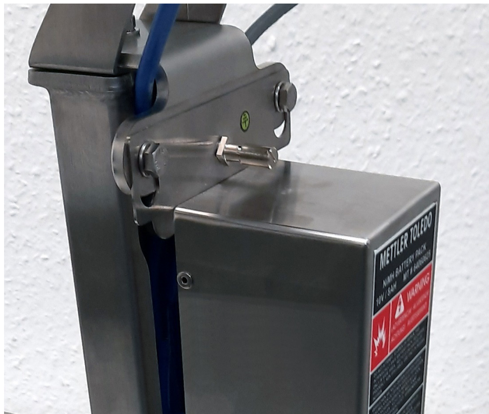
Figure 3-4: Battery Mounting Bracket, Installed
