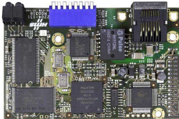
Figure 2-85: Ethernet / IP PLC Module
