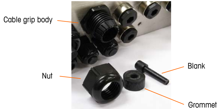
Figure 2-22: Cable Gland Components
