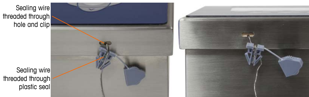
Figure 2-96: Harsh Enclosure Seal Threaded and Ready to be Closed – Standard Orientation (left) and with Panel Reversed (right)
