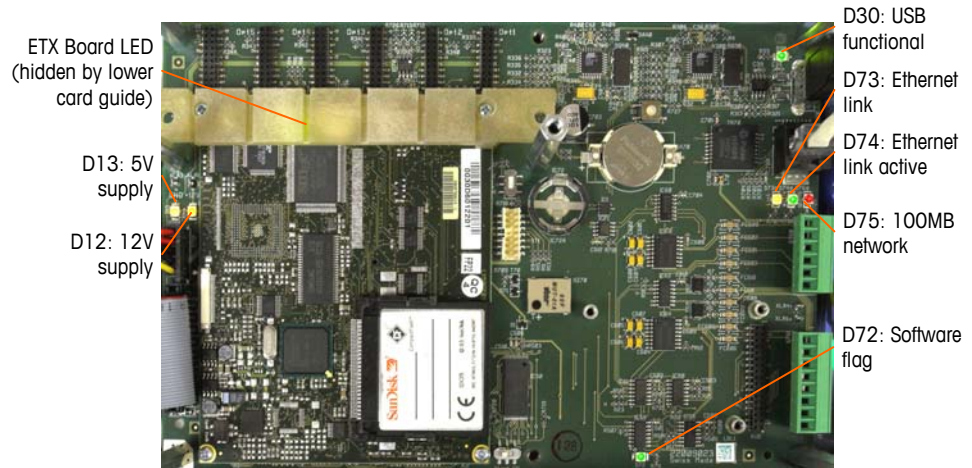
Figure 2-37: Main PCB LEDs
