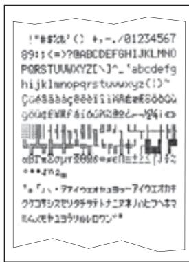
The RS-P42 is equipped with a self-test which automatically prints out the character set of the printer.
