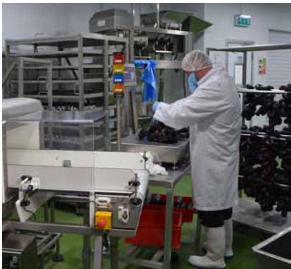
Traditional pudding rings are weighed and packaged in net bags before being inspected by a Profile Advantage metal detection system.
