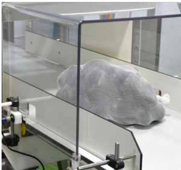
Traditional pudding rings are weighed and packaged in net bags before being inspected by a Profile Advantage metal detection system.
