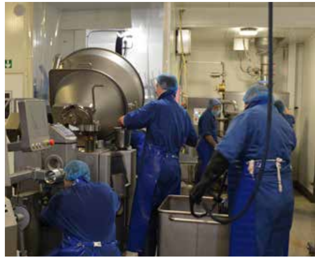
The HDS Pipeline system is fully stripped down for cleaning in between product changeovers.
