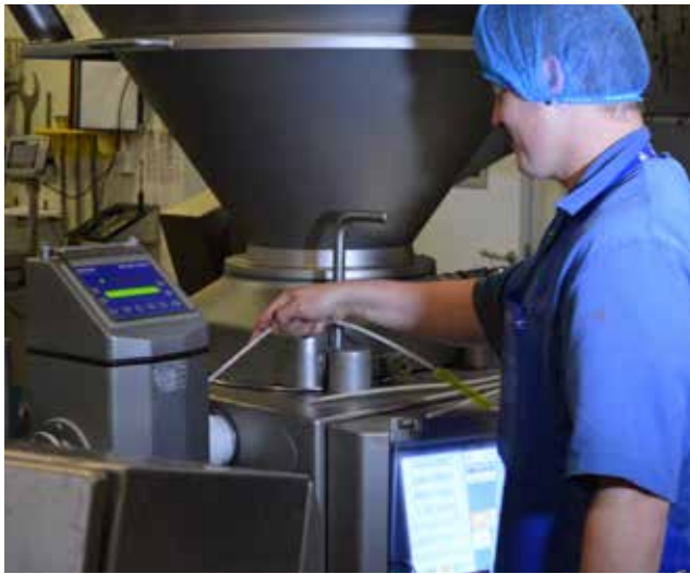
An HDS Pipeline system easily integrates with the Handtmann vacuum filler, inspecting pumped black and white pudding products immediately prior to vacuum filling.
