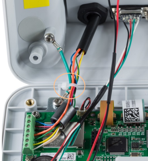
Figure 2-24: Analog Load Cell Pin Grounding and Ferrite Installation, IND231
