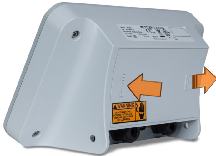
Figure 2-19: Removing the Battery Cover
