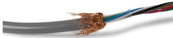
Figure 2-30: Load Cell Cable with Shield Wire Folded Back
