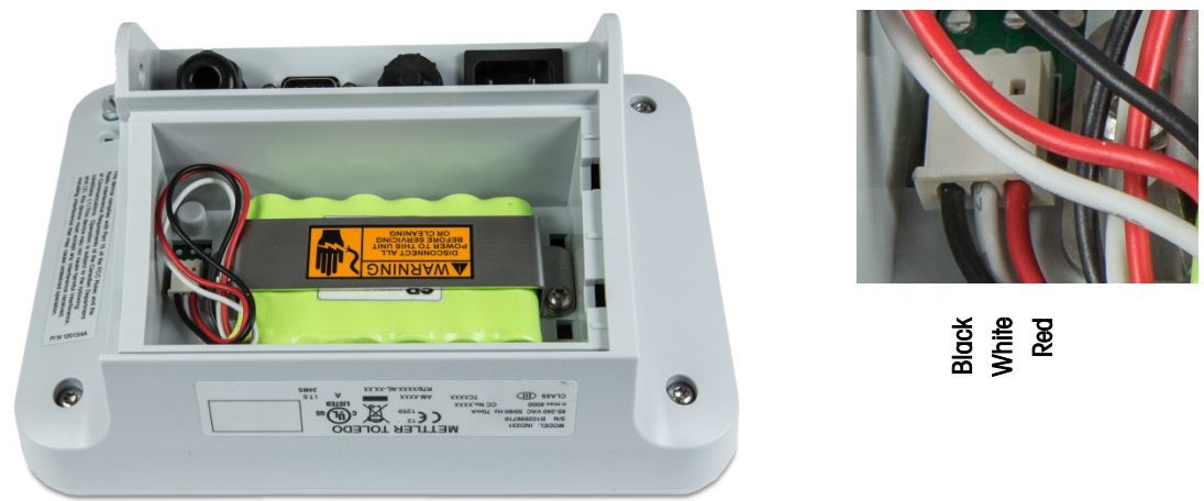
Figure 2-21: NiMH Battery Installed in IND231
