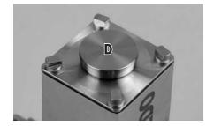
Put the **standard weighing pan** (D) onto the weighing pan adapter.
