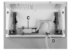
Feed the terminal cable through the cutout in the back of the terminal and plug in the jack (C). Make sure that the strain relief (D) is inside the terminal.
