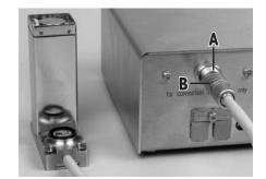
The weigh unit housing has no plug or socket but a direct cable exit. Typically, the cable length is 3 m.
