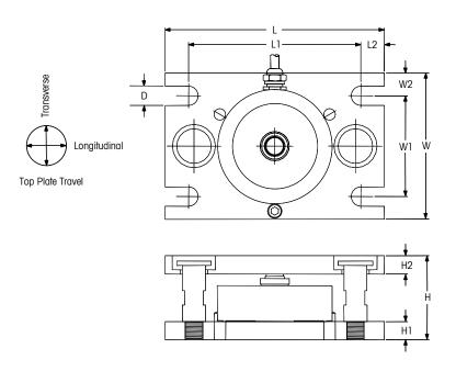
Note: Each weigh module is supplied with shipping/installation blocks to keep the top and bottom plates rigidly aligned during shipping and installation.
