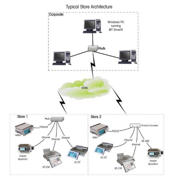
SmartX can be implemented in many configurations within your enterprise. The above diagram details one possible configuration for implementing SmartX across a network. Connections can be wired or RF. Scales can be all of the same family or from different product lines (and, in some cases, manufacturers!) and multiple users can communicate to the devices by utilizing the client/server capability of SmartX.
