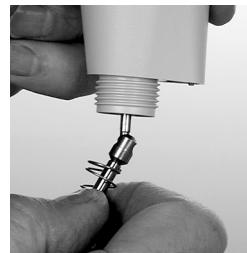
FIGURE 6C REPLACING THE LIQUID END (3)
