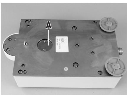
The hanger opening is on the bottom of the cell under a round cover (A).
