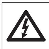
METTLER TOLEDO recommends that you use the AC adapter provided with your unit to operate it. Make sure that the voltage printed on the adapter matches your local power supply. Plug the adapter into a grounded outlet only.
