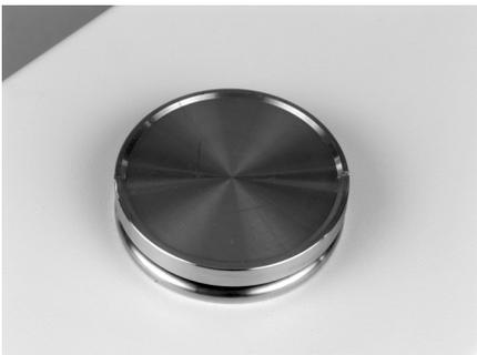
Place the weighing pan cone into the weighing pan retainer. You do not need to insert it in any specific position; the standard weighing pan will turn freely.
