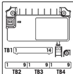
**Note:** This is a 4-wire-product with an active 4–20 mA analog output. Please do not supply to Pin1–Pin6 of TB2.
