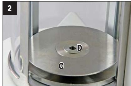
Lift off the intermediate shelf (C) and the sleeve (D).
