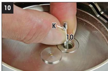
Insert the weighing pan fastener (10).
