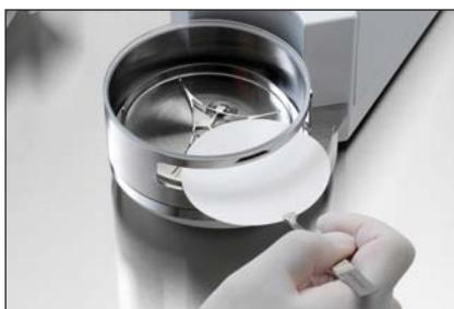
Insert the filter **sideways** through the opening in the draft shield.
