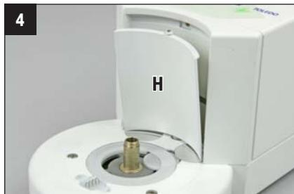
Remove the sealing cover (H).
