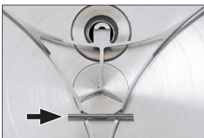
You can use the integrated weight or an external weight for testing or **adjusting the balance**.
