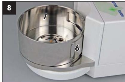
Insert the draft shield (7) and the sealing cover (6) and press them down. Turn the draft shield gently until it clicks into position (the sliding bushing (5) must sit in the slot on the underside of the draft shield).
