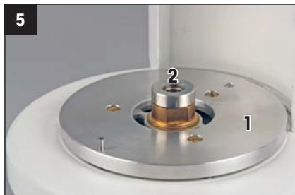
Insert the coupling (1) and screw on the positioning nut (2).
