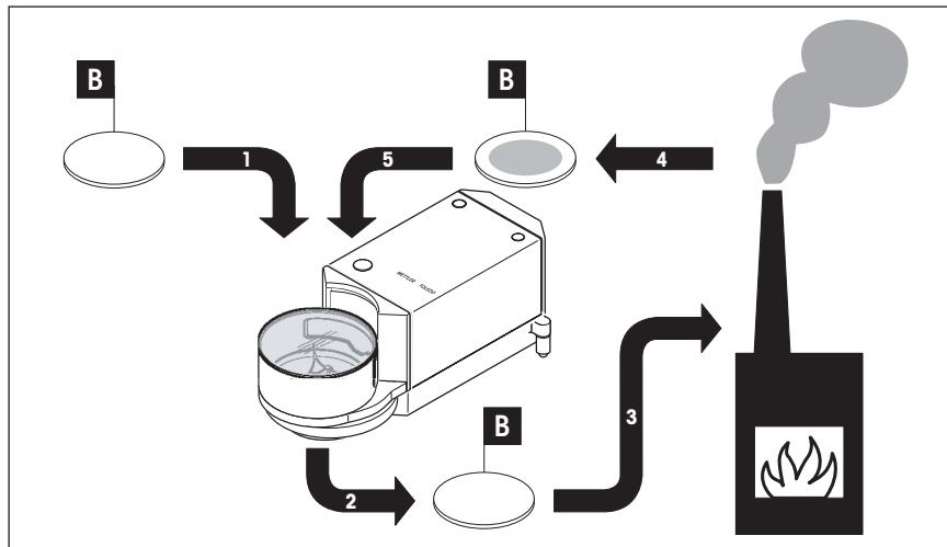
With the simple method, only one **test filter** (B) is used.
