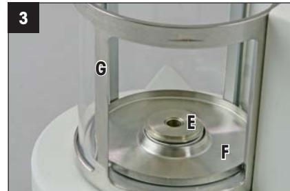
Unscrew the mounting (E), remove the drip pan (F) and lift off the glass draft shield (G).
