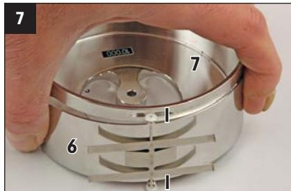
Attach and secure the sealing cover (6) to the draft shield (7). Ensure that the small wheels (I) sit in the slots of the draft shield.
