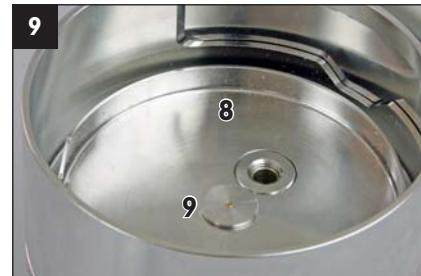
Attach the filter pan (8) and screw on the knurled nut (9). Test the function of the draft shield using the door operating buttons on the balance (open to the left and to the right).
