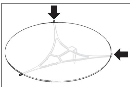
Place the filter **directly in the center**, so that it touches both vertical pins on the back cantilever arms of the filter weighing pan.
