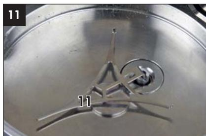
Attach the large or small filter weighing pan (11).
