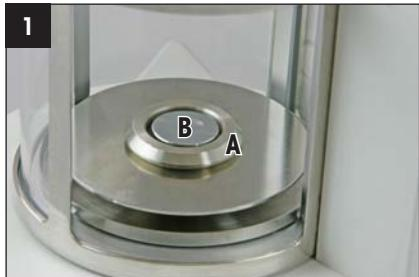
Lift off the draft shield ring (A) and the weighing pan (B).
