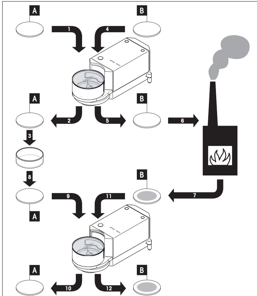
This method also allows for changes in ambient conditions and the potential contamination of the measuring room. Two filters are used for this, a **reference filter** (A) and a **test filter** (B).
