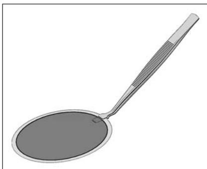
The filter set is supplied with specially designed **tweezers**. We recommend that only these tweezers be used for filter weighing. The upper tongue is shortened to ensure that the tweezers do not come into contact with the material on the filter. The lower, longer tongue ensures that the filter can be held steadily in the tweezers.
