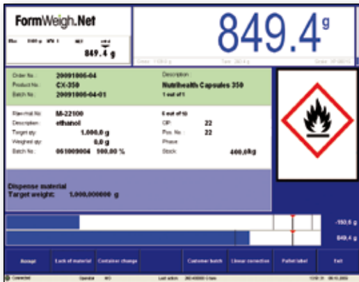
The FormWeigh.Net® weighing station software shows all key component information at a glance, including pictograms, such as hazardous symbols.
