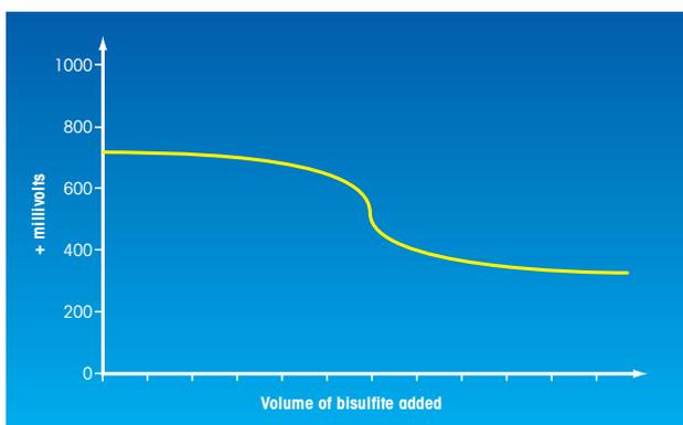
Continuous processes are controlled to operate near a single point on such a curve. The curve for a specific installation may be shifted significantly from these millivolt values but the basic shape will be similar for the dechlorination reaction. On-line experience is necessary at startup to establish the particular millivolt operating range and setpoint for an application
