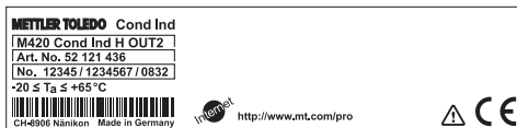
Fig.: M420 Cond Ind H OUT2 rating plate at outside bottom of front
