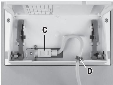
Feed the terminal cable through the cutout in the back of the terminal and plug in the jack (C). Make sure that the strain relief (D) **is inside the terminal**.
