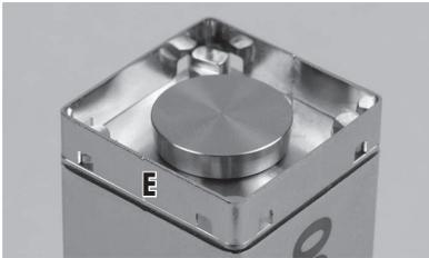
Slide the **draft shield** (E) onto the weigh unit by evenly pressing down on two opposite corners until it engages with an audible 'click'.
