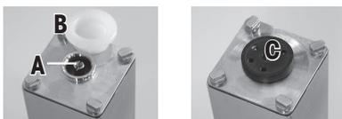
Remove the **white plastic cover** (B) from the weighing cell. This cover protects the **weighing pan support** (A) from damage during transport and keeps liquid from penetrating into the weighing cell during cleaning. Therefore keep the cover in a safe place!
