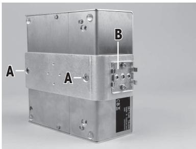
Remove the two existing screws from the bottom side of the electronic unit (Torx T-20) and use the provided Torx T-20 countersunk head screws (A) to secure the mounting bracket.
