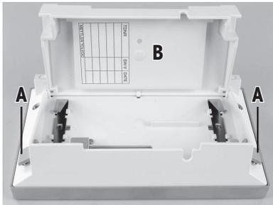
Place the terminal on a flat surface with the display face down. Press the two tabs (A) on the back of the terminal to open it, and open the bottom of the terminal (B).
