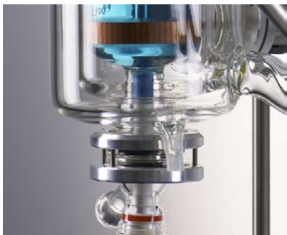
RTCal™ vessel with integrated heat flux sensors.
