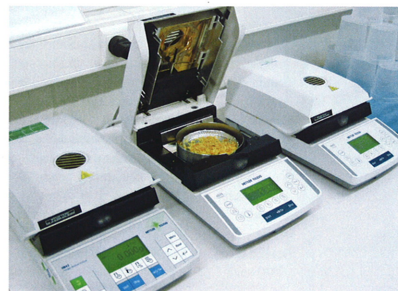
At the service of crispy tortilla chips: HB43 moisture analysers in the Poco Loco quality control laboratory.
