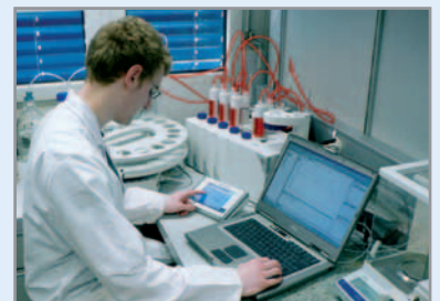
T90 – Rondo 20 - LabX pro titration system in production control for acid, base and saponification numbers for the analyses of a diverse range of lubricants.
