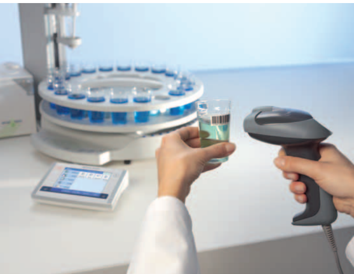
LabX pro titration controls the Compact Coulometric KF C30 – Stromboli oven sample changer system in a Quality Control lab for determination of the water content of lubricants.
