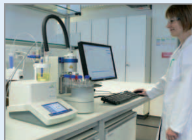
LabX pro titration controls the Compact Coulometric KF C30 – Stromboli oven sample changer system in a Quality Control lab for determination of the water content of lubricants.
