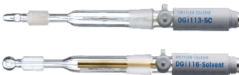
Figure 1: DGi113-SC and DGi116-Solvent, the special sensors for non-aqueous titrations.
