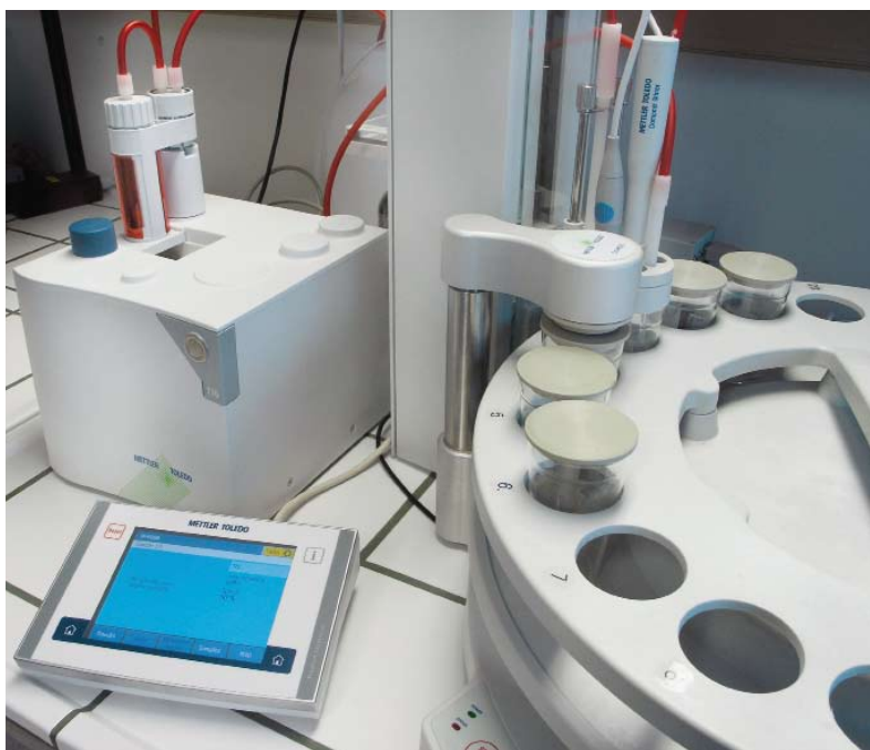
Figure 1: The Titration Excellence T70 with Rondo 20 sample changer and CoverUp™ lid handling unit.
