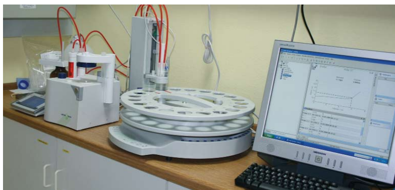
Figure 5: Standard hops analysis using a METTLER TOLEDO Excellence titrator, Rondo 20, and LabX titration.
