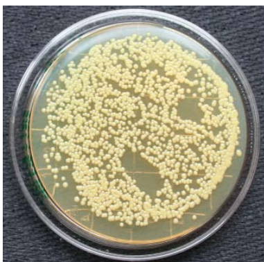
Figure 2: If cleaning is not completely effective, numerous colonies grow on the nutrient agar after incubation.
