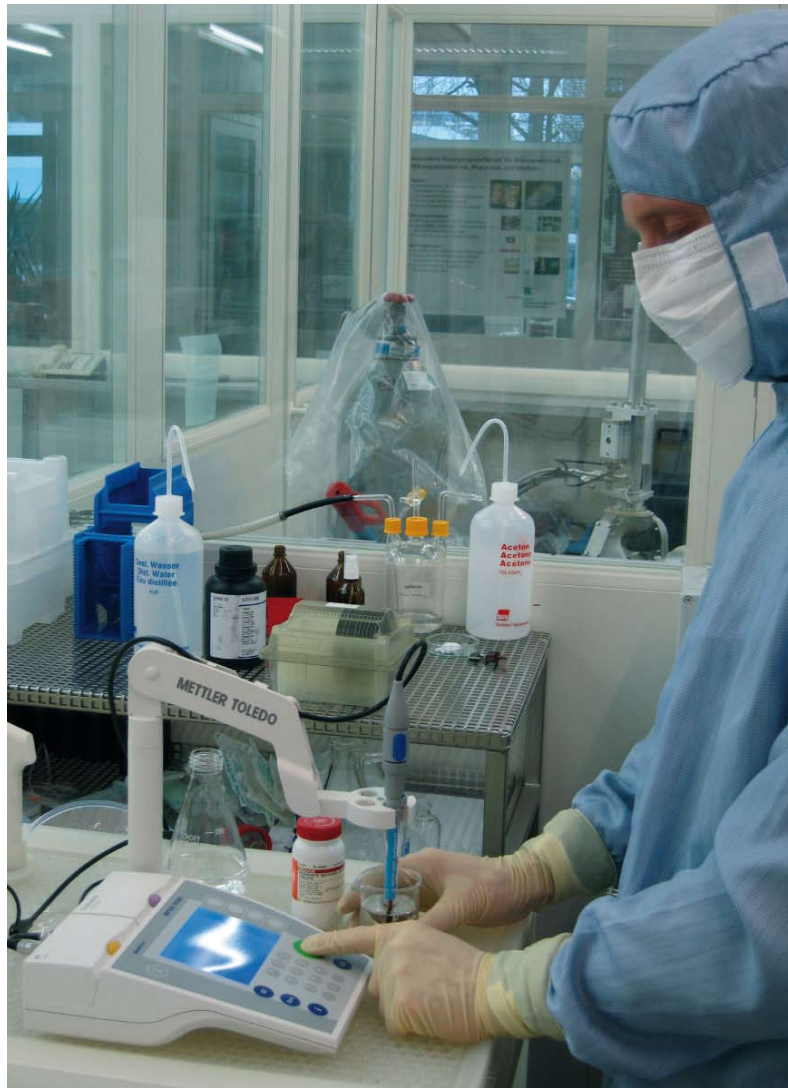
Figure 3: Markus Keller adjusts the pH of a potassium phosphate buffer using the SevenMulti™ S47. To reduce contamination, protective clothing and facemasks must be worn in the cleanest room in the world.
