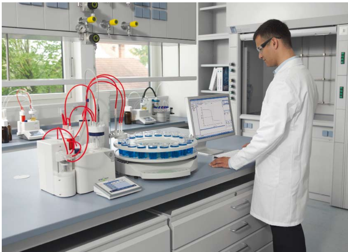
The automatic titration system in action: T90 Excellence titrator, Rondo 20 sample changer, Liquid Handler and LabX pro titration.
