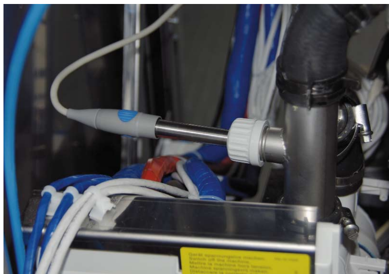
Figure 3: The InLab®741 is attached via a bypass next to the disinfectant's built-in online conductivity sensor.
