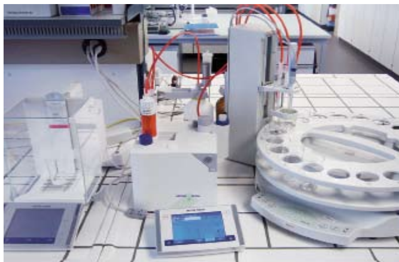
Figure 3: T90 Excellence titrator with Rondo 20 sample changer and Excellence analytical balance.
