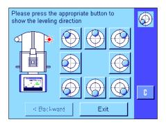
Watch the level indicator on your balance (this will light up when the level sensor is switched on) and press the button that matches the current position of the air bubble in the level indicator.
