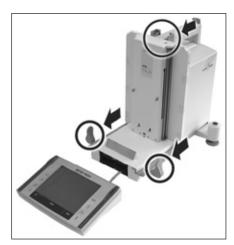
Push the guide of the upper draft shield door right to the front.
