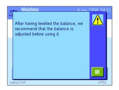
Before the balance returns to Weighing Mode, a message appears that advises you to adjust the balance after you have leveled it. Confirm the message with "**OK**".
