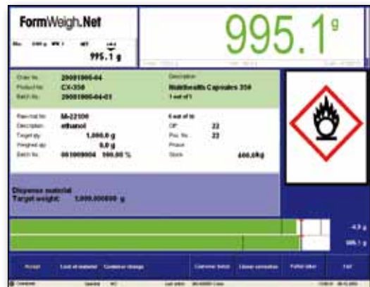
The real-time progress bar is clearly visible to the operator and changes its color according to the weighing progress.
