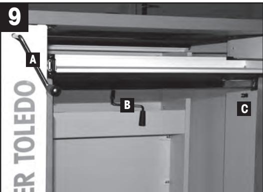
Use the two handles [A and B] to adjust both tables to an optimum ergonomic height. Then, clip the handle [A] into the respective holder [C].
