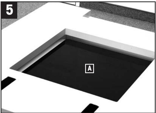
Carefully place the stone plate [A] in the balance table.
