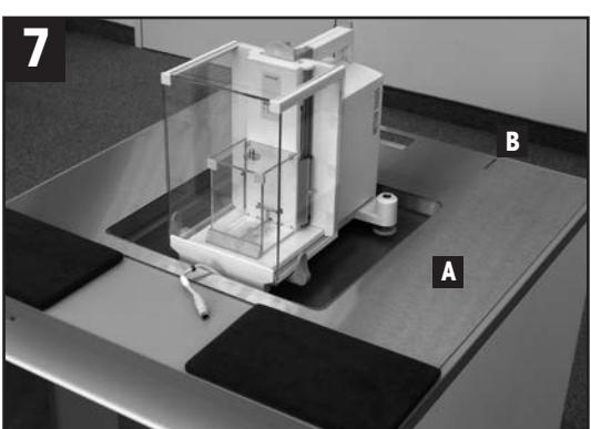
Place the balance, level it and connect it to the AC adapter. Place the metal sheet [A] and align the slots [B] with the recess in the working table.
