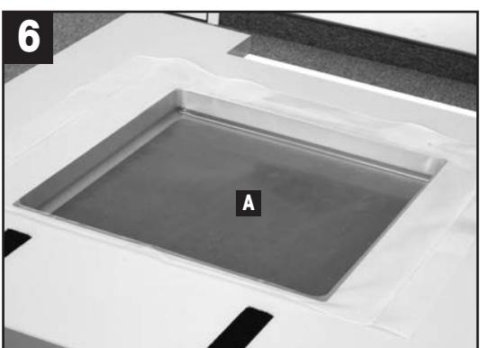
Place the flexible drip pan [A] in the working table. Adjust the height of the balance table (see step 5) so that the bottom of the drip pan is properly seated on the stone plate.
