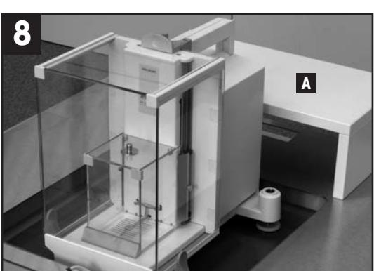
Install console [A]: Insert the two pins at the bottom of the console into the respective slots of the metal sheet (the console secures the metal sheet).
