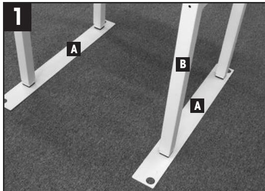
Choose an appropriate location (no vibrations, see balance manual). Locate positioning guides [A] and place balance table [B] (inner table) into the respective holes.
